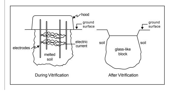
The heat used to melt the soil can also destroy some of the harmful chemicals and cause others to evaporate. The evaporated chemicals rise through the melted soil to the ground surface. Here, a hood, which covers the heated area, collects the chemicals. These chemicals are sent to a treatment system where they are cleaned up.
